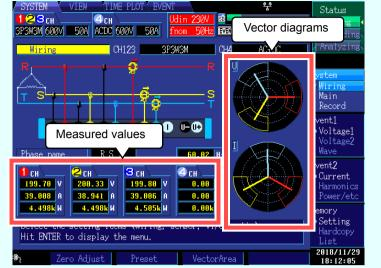
Verify that the connections are correct, referring to the vector diagrams and measured values on the [Wiring] screen.
